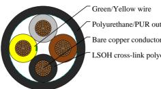
Polyurethane/PUR outer jacket Bare copper conductor LSOH cross-link polyolefin insulation
